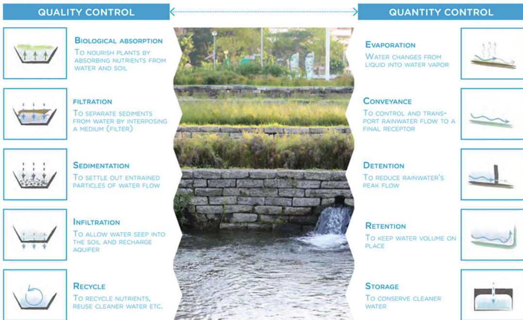
Water and Sustainable Design, Fig. 2 Both quality and quantity controls are key to rainwater collection, harvesting, and reuse. BGI Toolkit. (Credit: Giovanni Cossu (LCL Ramboll))
